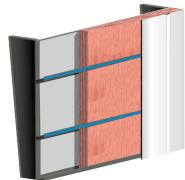
**b.** Faced Metal Building Insulation: Faced metal building insulation is a single layer of insulation that is rolled over the purlins and girts. This is sandwiched between the exterior cladding and the secondary to be held in place. This comes faced with WMP-50 Vapor guard.
